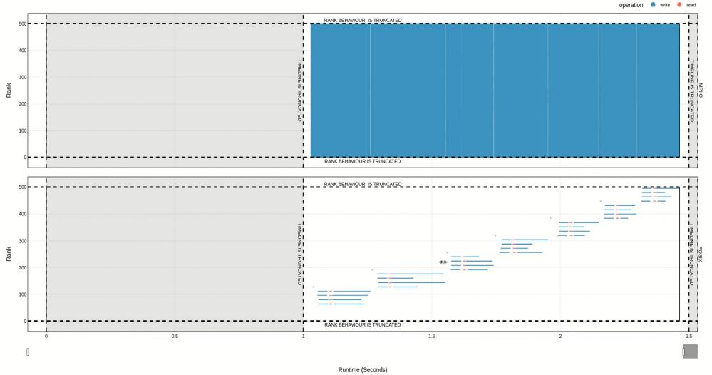
**Explore** the timeline by **zooming in and out** and observing how the **MPI-IO** calls are translated to the **POSIX** layer. Visualize relevant information in the context of each I/O call (rank, operation, duration, request size, and OSTs if Lustre) by hovering over a given operation.
