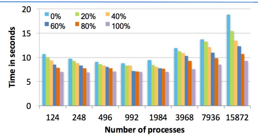
Write time with part of the data written to faster burst buffer and the remaining to slower Lustre file system on Cori.
