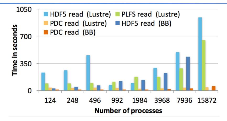
Total time for reading data of 5 timesteps from the BD-CATS-IO kernel from the Lustre and from the burst buffer. PDC is up to **11X** faster than PLFS and HDF5.
