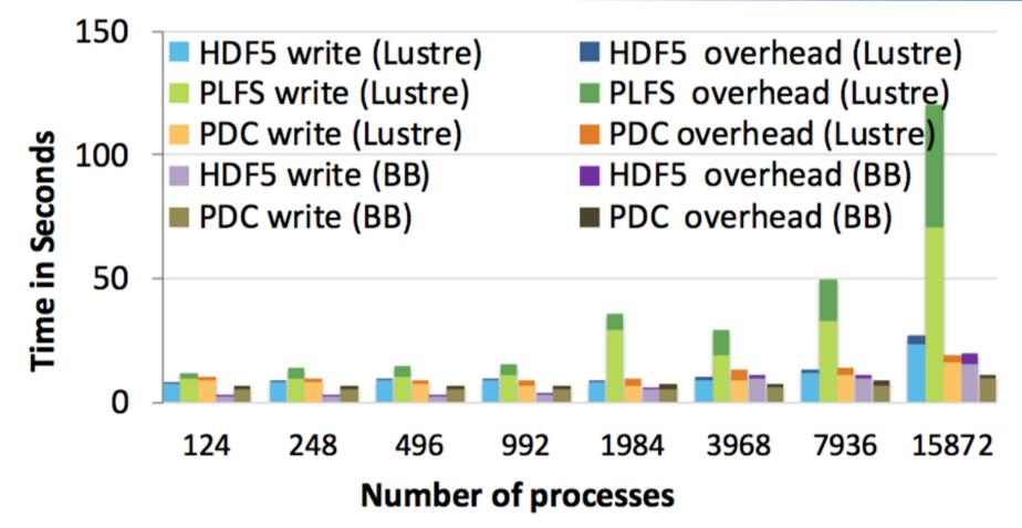
Total time for writing 1 timestep to Lustre and Burst Buffer using HDF5, PLFS, and PDC on Cori. PDC is up to 1.7x faster than HDF5 and 9.2x over PLFS
