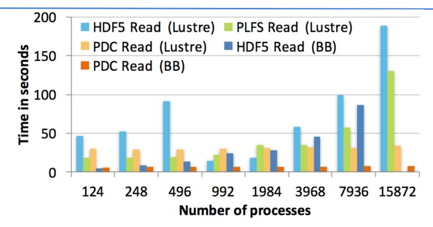
Total time for reading 1 timestep data using the BD-CATS-IO kernel using HDF5, PLFS, and PDC. PDC is up to 5x and 4x faster than HDF5 and PLFS.
