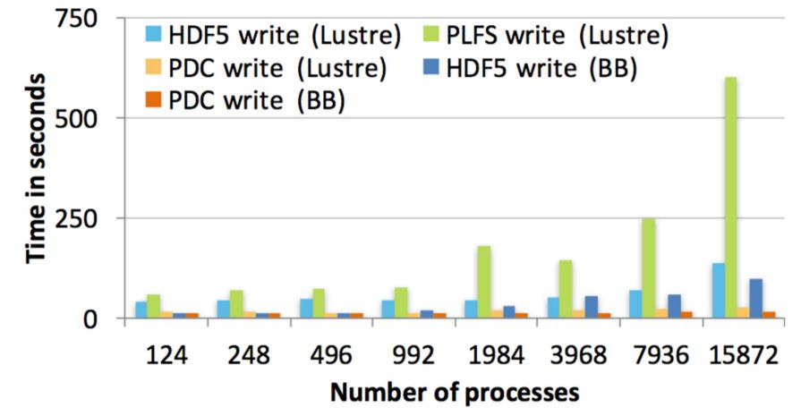
Total time to write 5 timesteps from the VPIC-IO kernel to Lustre and Burst Buffer on Cori. PDC is up to 5x faster than HDF5 and 23x over PLFS.
