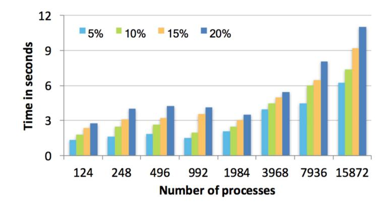
Time to read various selected object regions specified by the client processes from burst buffer on Cori.
