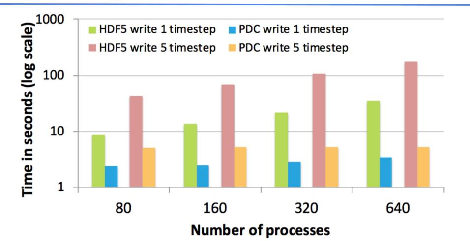
Total time to write 1 and 5 timesteps from the VPIC-IO kernel to the GPFS file system on Cooley. PDC is up to 7x and 35x than HDF5 to write 1 and 5 timesteps data.
