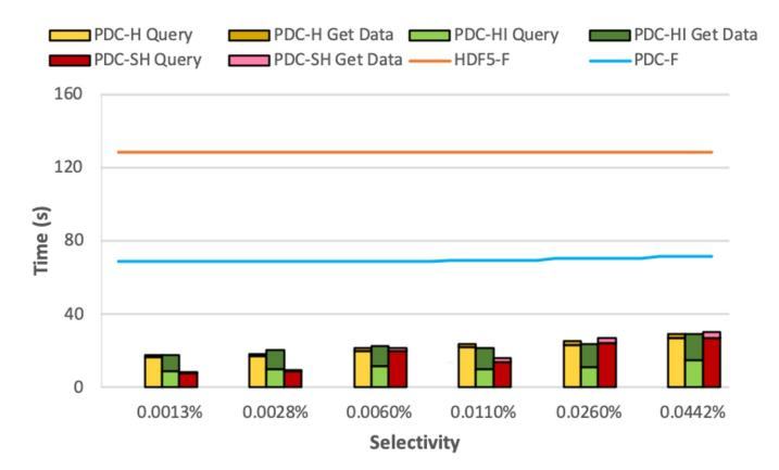
**PDC-H**: PDC with **H**istogram only, **PDC-HI**: PDC with **Hi**stogram and Fastbit Index, **PDC-SH**: PDC with **S**orted data (sorted by the 'energy' object) and **H**istogram. **HDF5-F**: amortized time to evaluate the 6 queries with HDF5 **F**ull scan. **PDC-F**: amortized time to evaluate the 6 queries with PDC **F**ull scan.
