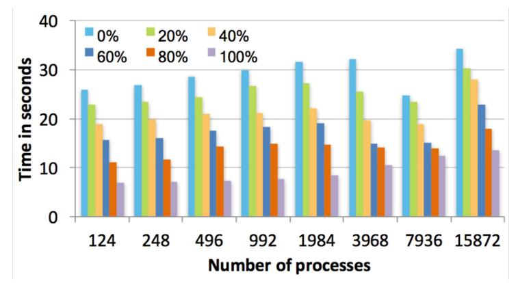
Read time with part of the data written to faster burst buffer and the remaining to slower Lustre file system on Cori.
